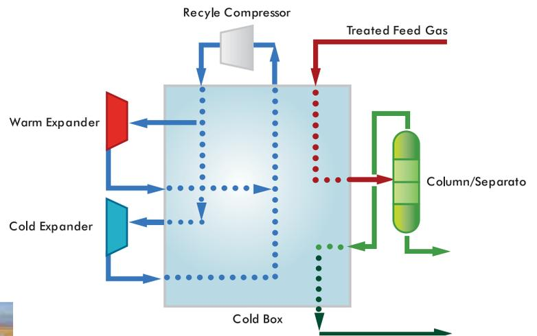
Figure 3 – Cosmodyne's Natural Gas Liquefier Nitrogen Cycle
