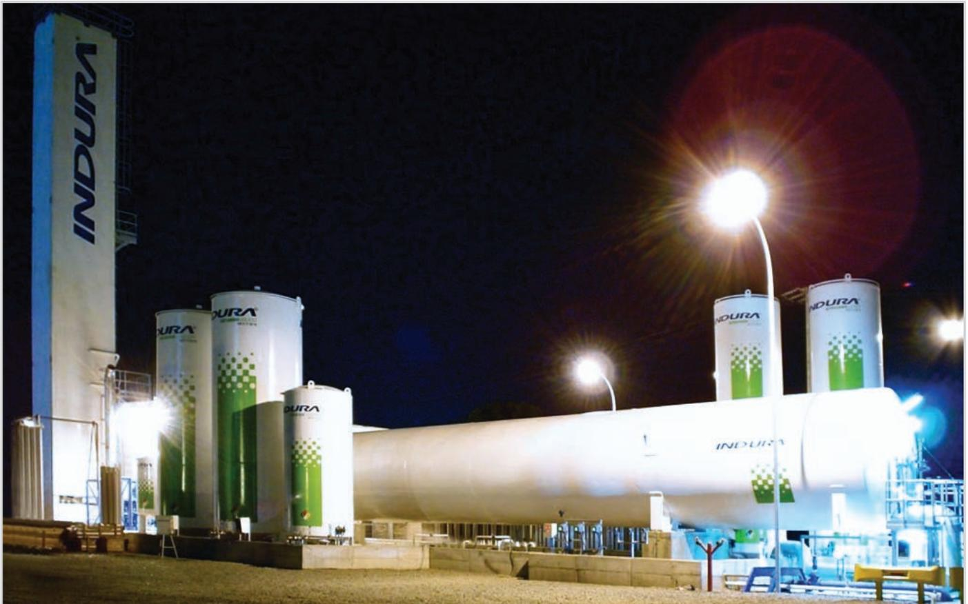
In 1998, a Cosmodyne Aspen 1000 embarked on a South American odyssey that would span a length of five years. The high efficiency, modular air separation plant was purchased in 1996 by Indura, Chile's leading industrial gas company. Designed to cost-effectively produce liquid oxygen, liquid nitrogen, liquid argon, and gaseous nitrogen, the Aspen plant met the growing air separation needs of South America.
