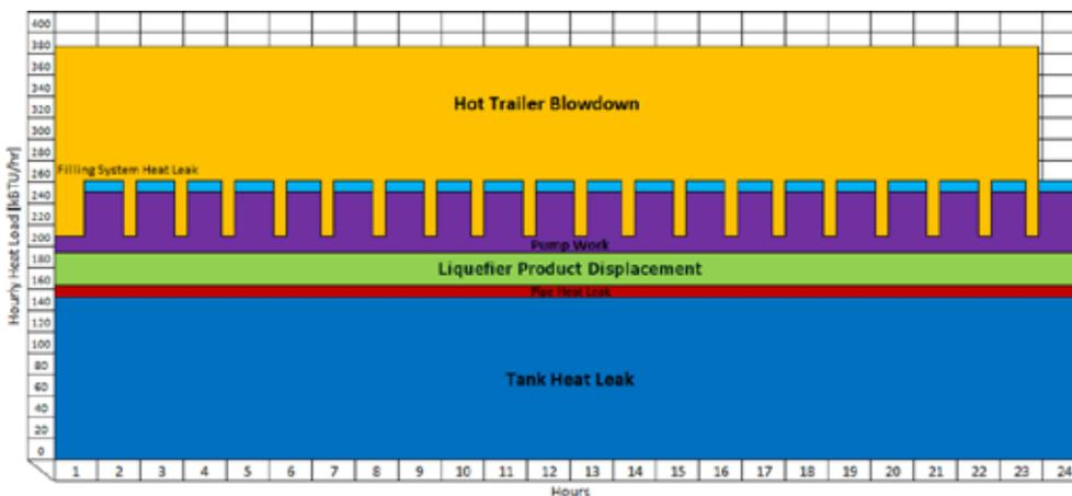
**Figure 2.** Example daily schedule of expected heat loads when filling 20 high pressure 10 000 gal. trailers.
